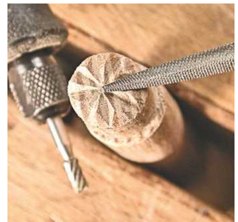
▲ Pic. 10 To complete the tool cuts, Jeff used the corners of a square file
